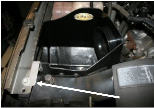
8. Install the CAB assembly into the vehicle where the factory airbox used to be using three 6mm hex bolts (#12) and three flat washers (#11) thru the bottom. Now reinstall the factory fender bolt thru the bracket and into the fender. Adjust the assembly for fit and tighten all bolts and nuts at this time. Apply the Airaid Foil Decal onto the Panel as shown.
