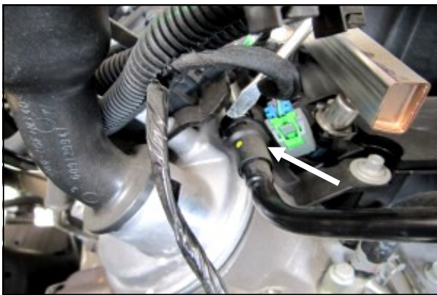
4. Remove the plastic PCV breather line from the factory hard line. A standard screwdriver works well for depressing the locking tab in the coupling.
