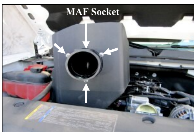
8. Install the Filter Adapter (#4) onto the Cold Air Box or CAB (#3) as shown using the three 1/4-20 Button Head Screws (#10) and 1/4" Flat Washers (#11). Note: The MAF socket is to be in the 12:00 position when properly assembled.
