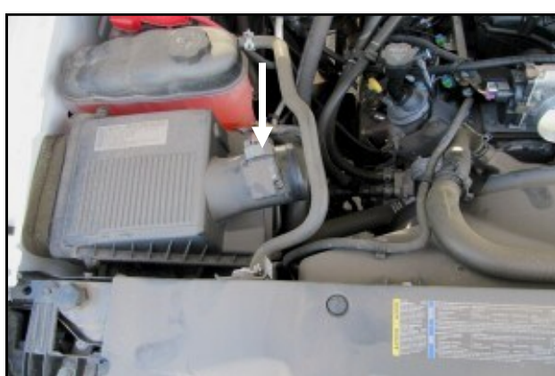
5. Disconnect the Mass Air Flow or MAF sensor and remove the factory airbox from the vehicle. The airbox is secured to the vehicle with grommets and simply lifts out.
