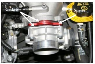
**4.** Install the Poweraid Spacer between the throttlebody and the intake manifold with the first supplied gasket next to the intake manifold, and the second supplied gasket next to the throttlebody as shown. Make sure the "flow" arrow printed on the spacer is pointing towards the intake manifold. Install the provided bolts and washers thru the throttlebody and
