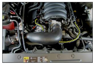
9. Install the Intake Tube and tighten the Clamps. Connect the new breathers to the Barbed Fittings in the Intake tube and the Quick Connect Fittings to the Valve covers.
