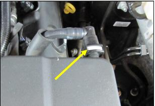
2. The quick connects for the valve cover breathers are removed by depressing the grey locking tab in the fitting and sliding them off.
