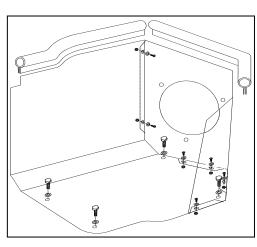
**6.** Assemble the Airaid Cool Air Dam panels (#2, #3) using five 6-32x 5/16" screws (#9), #6 flat washers (#10), and 6-32 keps nuts (#11).
