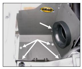
7. Install the air filter adapter (#4) using three ½-20x ½" button head bolts (#12), and 1/4" flat washers (#13). Position the Airaid Cool Air Dam in place of the factory airbox & secure it with four M6-1x25 hex bolts (#14) and 1/4" flat washers (#13). Apply the Airaid Decal as shown.
