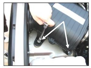
**2.** Using a 10mm socket, remove the three bolts that secure the factory airbox to the inner fender (save for reuse).
