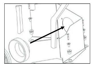
**5.** Install the filter adapter (#4) into the Airaid Cool Air Dam using three 1/4-20x 5/8" bolts (#6), and 1/4" flat washers (#7).
