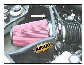
**8**. Install the Airaid Premium Filter (#1) onto the filter adapter, and tighten the hose clamp. Install the provided weather strip (#5) onto the top edge of the panel. Apply the Airaid Foil Decal onto the Panel as shown.
