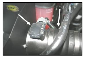
**10.** Reinstall the **MAF** sensor onto the filter adapter using two 8-32 x 5/8" Allen Bolts (#13). **Do Not Use The Factory Screws!**
