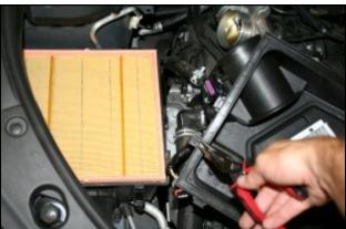
**4.** I urn the factory airbox lid over and locate the wire harness anchor. Using a pair of needle nose pillars, compress the ribs of the anchor and remove it. Remove the factory air filter and set it aside.
