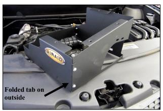
5. Join the two Airaid panels together with the ioided tabs on the outside, using the four 6-32 screws (#15), #6 Flat washers (#14), and #6 Keps Nuts (#13). Apply the Airaid Foil Decal onto the Panel as shown.
