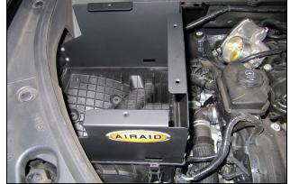
**6.** Slip the Alraid Panel tabs into the slots in the factory airbox and partially install the Panel assembly onto lower half of the factory airbox as shown. Do not latch the airbox clips at this time.
