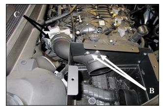
9. A) Insert the Filter end of the Intake Tube into the Panel assembly opening and guide the Coupler side onto the throttle body. B) Rotate the Intake Tube until the mounting holes are aligned with the Panel holes. Secure the Intake Tube to the panel assembly using the two 8-32 button head screws (#16). C) Tighten the Hose Clamps, and fasten the airbox clips at this time.
