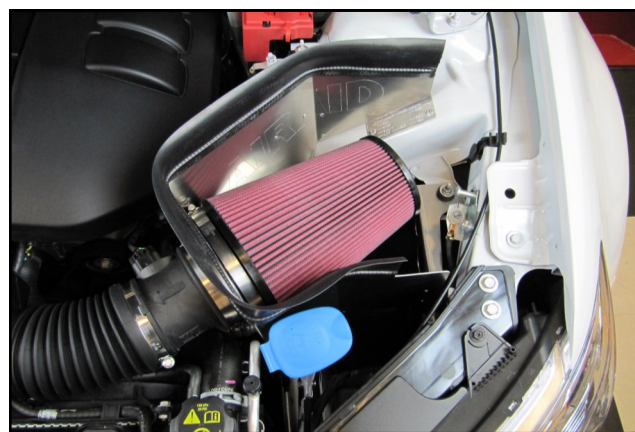
20. Install the Weatherstrip onto the top edge of the Air Dam with the contour rolling away from the Filter.
