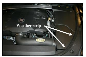
15. A) Install the 11" Weather Strip (#11) onto the curved edge of the top cover (#6) and install the top cover onto the Airaid filter box using the four 1/4-20 Black screws.(#22). B) Line up the intake bracket with the fender bolt hole, and secure the assembly using the factory bolt. Reinstall the Factory engine and shock tower covers .Note: These steps must be performed in order to avoid difficulty with bolt hole alignment.
