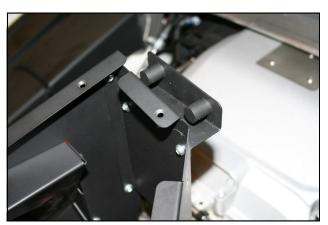
7. Attach the OEM Cover Bracket (#7) to the Rear Panel a shown using the remaining two sets of 6-32 hardware
