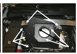
**9A)** Install the Filter Adapter onto the MAF panel using three 1/4-20 Button Head screws (#18) and 1/4" Flat washers (#17). **B)** Attach the Weather Strip (# 11) to the curved edge of the MAF Panel. **C)** Insert the 5/8" hose anchors (#30) into the two horizontal tab holes on the MAF panel.
