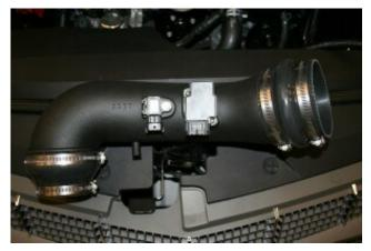
10. Transfer the air sensors from the Factory air box lid into the Airaid intake tube(#2). Do not use factory hardware! Secure the MAF sensor using the two #8-32x 1/2 screws (#16) and Lock Washers (#17), and the MAP sensor with the 1/4-20x3/4 bolt (#19).Install the Reducer Coupler and one #64 clamp(#26) and the #48 (#27) clamp on the 90 deg bend of the Intake Tube. Install the Hump Hose (#9) and 2 #64 clamps(#26) on the opposite end of the Intake Tube.
