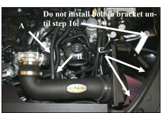
**14. A)** Replace the factory breather line on the valve cover with the 26" Airaid Breather Hose(#12). **B)** Secure the breather hose to the intake tube nipple using the black Speed Clamp (#32).**C)** Slide the Edge Clip Cable Ties (#31) about 6" apart along the fender pinch weld and return the coolant line to it's original location. Secure the coolant line using the cable ties and trim off
