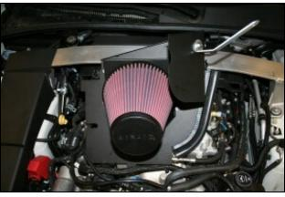
**11.** Install the Bracket (#28) on to the Rear Panel (#3) as shown using one 1/4-20 Button Head Screw (#17), 1/4" Flat Washer (#20), and 1/4" Serrated Nut(#21). Complete the assembly by attaching the Airaid Premium Filter (#1) to the Filter Adapter (#10).
