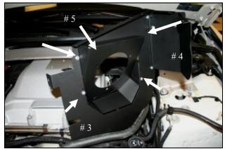
**5.** Install the Adapter Panel (#5) to the MAF Panel (#3) as shown using four 6-32 screws (#12), 6-32 Kep nuts, and #6 flat washers (#14). Attach the Rear panel (#4) to
