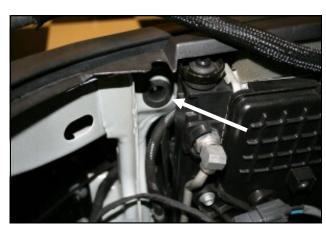
**4.** Use caution not to loose the factory core support grommet while removing the airbox assembly. It will be used in step 11.
