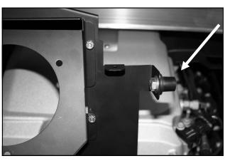
7. Attach the 5/8" Well Nut (#23) to the vertical MAF Panel tab as shown using the 5/16 Hex Bolt (#21) and the 5/16" flat washer (#22).
