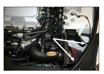
12. Install the Airaid Intake Tube (#2) assembly onto the filter Adapter first, and then onto the throttlebody. Adjust for fit, and tighten all 3 hose clamps. Next reconnect the MAF sensor and Breather line. Slide the Edge Clip Cable Ties (#30) about 6" apart along the fender pinch weld and return the coolant line to it's original location. Secure the coolant line using the cable ties and trim off excess.
