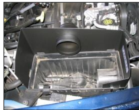
7. Mount the Airaid Cool Air Dam in place of the original air box lid & snap into place.
