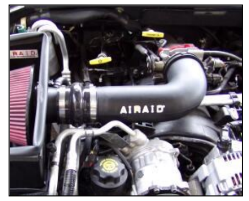
8. Mount the Airaid Premium filter inside the Cool Air Dam and secure with hose clamp provided. Apply the Airaid Foil Decal onto the Panel as shown.
