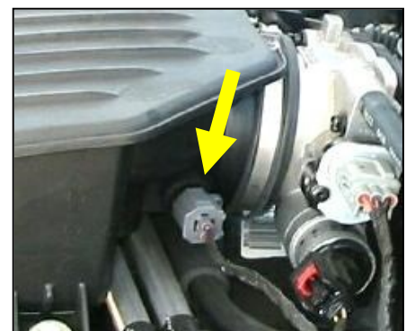
4. If your vehicle is equipped with an air temperature sensor, disconnect and remove the sensor & retain for later installation with Airaid kit.
