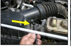
**2.** Unhook vacuum line from airbox, and remove from vehicle at the canister below the master cylinder. (Save for later use.)
