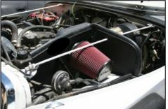
**18.** Install the Airaid Premium Filter and the weather strip on the CAD, as shown. (Hint: start the weather strip near the radiator support and work towards the back of the vehicle.)
