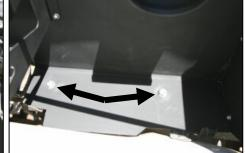
**10.** Install two <sup>1</sup>/<sub>4</sub>"-20 bolts and washers thru the top, and fender washers and nuts on the bottom, where the factory grommets were removed
