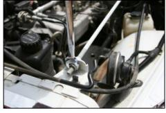
**8.** Using a 9/16" wrench, loosen the nut on the radiator rod support, and lift it up.
