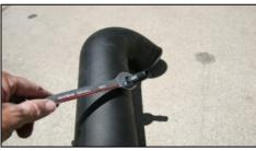
**14.** Install the ½" barbed fitting into the intake tube.
