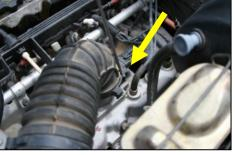
**3.** Pry open the plastic clamp that holds the factory intake tube to the throttle body. Unhook the 3 metal latches on the airbox that hold it to the mounting plate, and remove the intake assembly.
