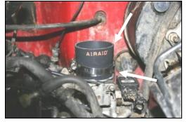
**17.** Install the reducer (#6) onto the throttle body using two #44 hose clamps (#16). Tighten <u>only</u> the hose clamp on the throttle body for now..
