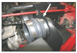
**16.** Install the hump hose (#5) onto the back side of the **CAD** tube using two #72 hose clamps (#17). Tighten <u>only</u> the hose clamp on the metal tube for now.
