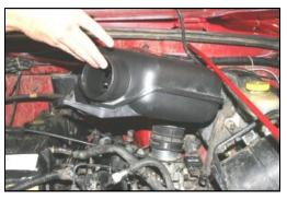
6. Remove the resonator from the vehicle.
