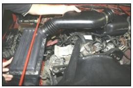
**2.** Unlatch the clips on the factory air cleaner lid, next remove the lid, and tube as an assembly.
