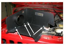
11. Assemble the two Cool Air Dam panels (#2) & (#3) using the four 6-32 screws (#8), #6 flat washers (#9), and nuts (#10).Apply the Airaid Foil Decal onto the Panel as shown.
