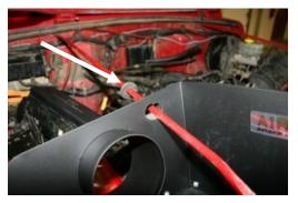
**12.** Slide the rubber grommet (#19) over the radiator support, followed by the assembled **CAD.** Use caution not to scratch the paint on the support rod.
