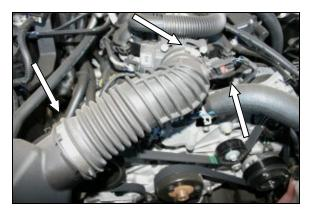
1. <u>Disconnect the negative battery cable!</u> Loosen 2 hose clamps on each end of the factory intake tube. Slide the red locking tab, and then squeeze the black tab, and disconnect the intake tube temperature sensor wiring harness. Remove the tube from the vehicle.
