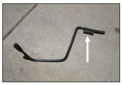
13. Remove the factory hose from step 2, and install the new 3/8"x4" hose (#23) on the end of the vacuum line as shown. Re-install the vacuum line. (Refer to step 2.)
