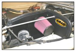
**18.** Install the Airaid Premium Filter (#1)and the weather strip (#9) onto the **CAD**, as shown. Apply the Airaid Foil Decal onto the Panel as shown.
