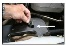
**4.** Remove the two grommets from the airbox mounting plate.
