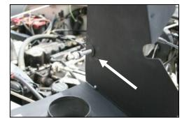
7. Assemble the Cool Air Dam (CAD) panels (#2, #3, & #4) as shown using the 5 provided screws (#10), washers (#11), and nuts (#12).
