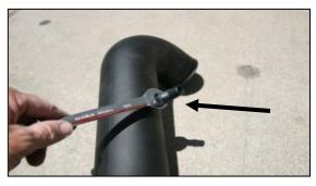
14. Install the  $\frac{1}{4}$ " barbed fitting (#22) into the intake tube.
