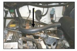
17. Replace the factory breather hose with the  $\frac{1}{2}$ "x 14" breather hose (#8) between the valve cover and the intake tube using two #16 speed clamps (#21) as shown.
