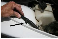
6. Carefully remove the wire loom clamp from the hole in the inner fender. Use caution not to damage the clamp, as it will be reused.
