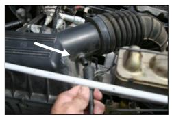
2. Disconnect the vacuum line from the airbox and at the canister below the master cylinder. (Save for reuse.)
