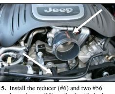
15. Install the reducer (#6) and two #56 hose clamps (#9) on the throttle body as shown. **Do not tighten** the clamps at this time. Secure the breather hose to the air conditioner line using the supplied zip tie (#15).
