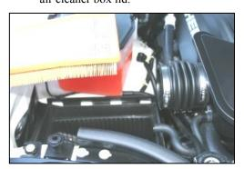
**4.** Remove factory air filter from the air cleaner box.
