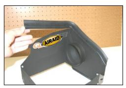
**12.** Install the weather strip (#7) on the top of the Quick Fit assembly. (Hint: start at one end, and go towards the other end, don't start in the middle.)
