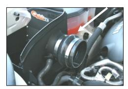
14. Install the hump hose (#5) and two #60 hose clamps (#10) on the Quick Fit assembly.Do not tighten the clamps at this time.
