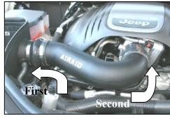
18. Carefully install the end of the Airaid Intake Tube (#4) into the hump hose, and then into the reducer on the throttle body as shown. Adjust the tube as needed, and then tighten the four hose clamps.
