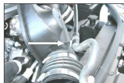
**9.** Slide the clip off of the resonator that holds the breather tube in place.
