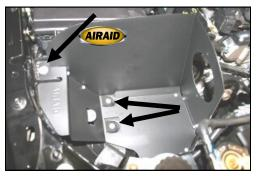
12. Install the CAD into the vehicle. Install the two 3/8 x1 1/4" button head bolts (#13), thru the bottom panel, and into the well nuts. Reinstall the factory bolt removed in step #7 thru the panel, and into the fender well. Tighten all three bolts at this time.
