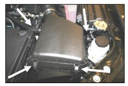
**3.** Unlatch the 4 metal clips that hold the factory air cleaner lid to the base. Next disconnect the breather hose that attaches to the rear of the air cleaner lid.
