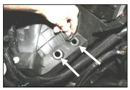
6. Remove the 2 lower grommets from the factory plastic air cleaner mount.
