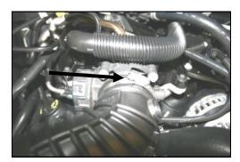
2. Loosen the intake tube hose clamp on the throttle body.
