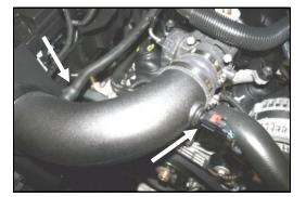
**17.** Very Carefully reinstall the temperature sensor removed in step #1, into the grommet in the Airaid Intake Tube. Reconnect the factory breather hose to the nipple on the intake tube.
