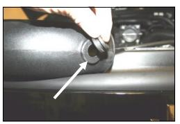
**14.** Install the supplied grommet (#17) into the Airaid Intake Tube (#2).
