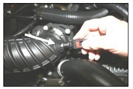
1. Disconnect the negative battery cable. Very Carefully remove the temperature sensor from the factory intake tube by using a circular motion while pulling it straight out. There is no need to disconnect the wiring harness.
