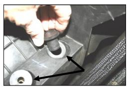
7. With a 10mm socket, remove and save the bolt from the factory plastic air cleaner mount. It will be re-installed in step #12.
