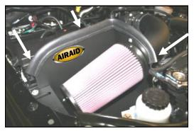
**18.** Install the Airaid Premium Filter (#1) onto the intake tube, and tighten the clamp. Next install the weatherstrip (#6) onto the top of the **CAD** as shown.
