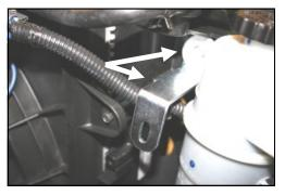
**10.** Insert the bolt, removed in step #8, thru the round hole in the provided L-bracket, and back into the radiator support. Leave the bolt slightly loose for now.
