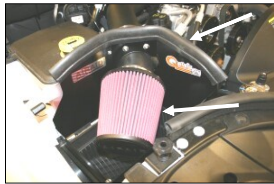
17. Install the Airaid Premium Filter (#1) onto the air filter adapter. Next, install the weather strip (#8) on the top of the Quick Fit panels as shown.
