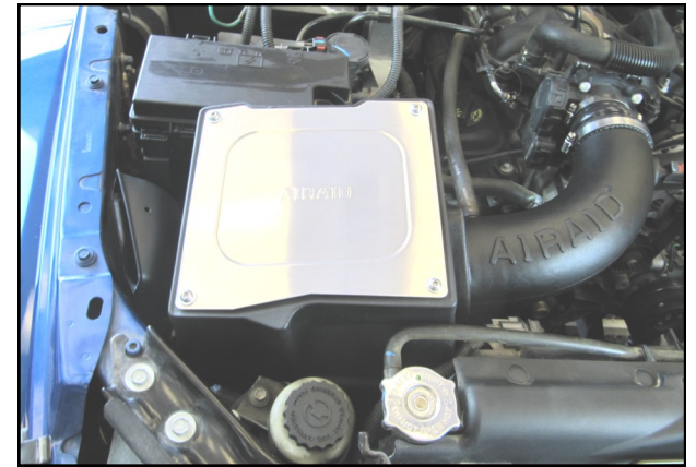
18. Double check your work! Make sure there is no foreign material in the intake path. Make sure all clamps, hoses, bolts, and screws are tight. Double check the hood clearance! Reconnect the negative battery cable!
