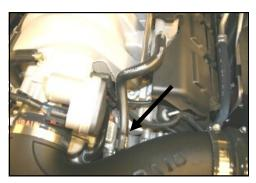
**16.** Re-connect the factory breather tube to the Airaid Intake Tube as shown.
