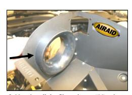
**8.** Next install the filter adapter (#6) using three ½ - 20 button head bolts (#12), and ½" flat washers (#13).
