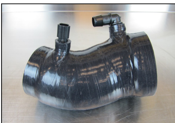
8. Transfer the air temperature sensor from the factory intake tube into the Airaid Intake Tube.
