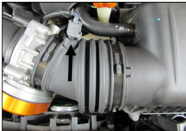
2. Disconnect the air temperature sensor. Loosen the throttle body clamp on the factory intake tube.
