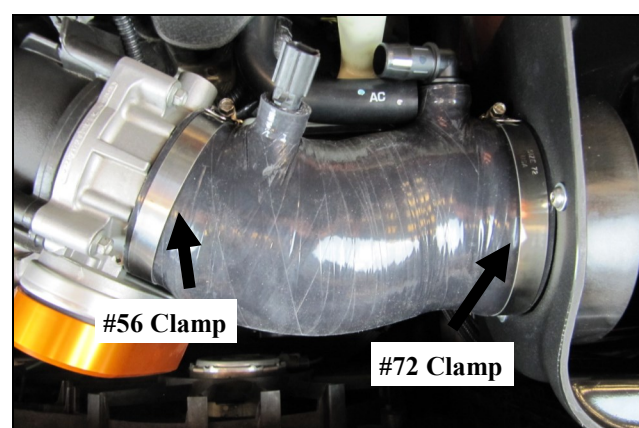
9. Place the #56 and #72 Hose Clamps onto the Airaid Intake Tube and install the assembly leaving the hose clamps loose for now.
