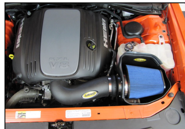
18. Reinstall the engine cover and oil cap. Reconnect the negative terminal on the battery.
