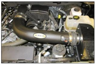
**9. A.)** Insert the Airaid Intake Tube into the couplers as shown. Check for alignment, and tighten all clamps. **B.)** Re connect the Mass Air Flow Sensor.
