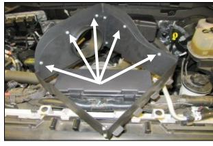
**5. For F-150 models only:** Fasten the Extension panel (#5) to the outside of the panel assembly using the remaining 6-32 screws, flat washers, and kep nuts.
