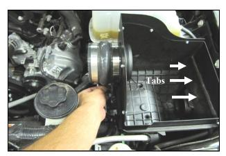
**6. A.)** Install the Silicone Hump Hose (#7) and two #64 Hose Clamps(#14) onto the Quick Fit assembly. Leave the clamps loose for now.
