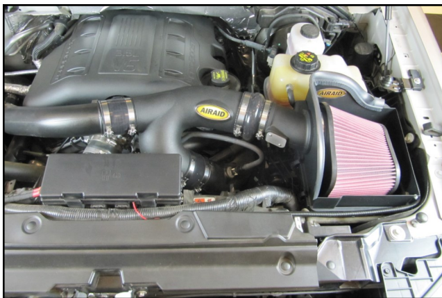
16. Double check your work. Make sure there is no foreign material in the intake path. Make sure all clamps, hoses, bolts, and screws are tight. Double check the hood clearance. Reconnect the negative battery cable.
