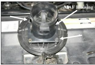
5. Remove the bolts that secure the MAF sensor housing to the adapter. Separate the adapter plate from the MAF sensor housing and save the sensor and housing for reinstallation in step #7.
