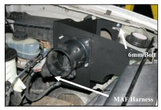
10. Install the CAD assembly into the vehicle using two 1/4-20x7/8" bolts (#15), four 1/4" flat washers (#16), one MAF backing plate (#19), and two 1/4" nylock nuts (#17). Leave the two bolts slightly loose for now for final adjustment. Refer to the line drawing on page 1 for reference. Next, reinstall the 6mm bolt thru the CAD, radiator overflow tank, and into the fender well. Reconnect the MAF sensor wiring harness.
