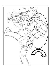
**15.** <u>4.6L engines</u>: Rotate the resonator box 90 degrees to provide clearance for the 3/4 x 12" L-hose (#7). Install the 3/4"x12" L-hose (#10) onto the Airaid Intake tube and the resonator box and secure it using the two #22 speed clamps (#23).
