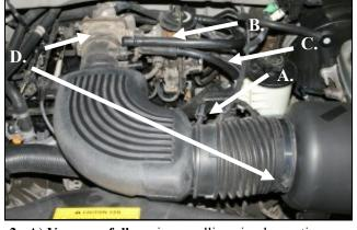
2. A) Very carefully, using a pulling circular motion, remove the air intake temperature sensor from the air intake tube. B) Disconnect the upper hard plastic tube from the air intake tube. C) Disconnect the crankcase breather at the intake tube and the valve cover, and remove it from the vehicle. **D**) Loosen two hose clamps and remove the air intake tube from the vehicle.
