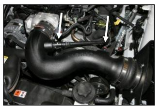
13. Install the intake tube assembly into the hump hose first, and then into the throttlebody coupler. Adjust for fit, and then tighten the three remaining hose clamps. Next, reconnect the MAF sensor wiring harness and lock the red tab. Now reconnect the factory breather tube to the factory fitting.
