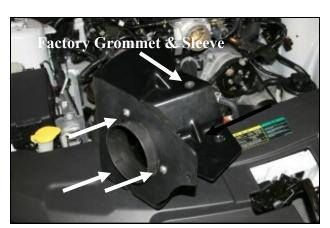
**8.** Install the filter adapter into the Cool Air Dam (#6) using three 1/4-20 button head bolts (#8), and three 1/4" flat washers (#9) as shown. Next install the factory grommet and steel sleeve removed in step #3 into the hole in the **CAD**.
