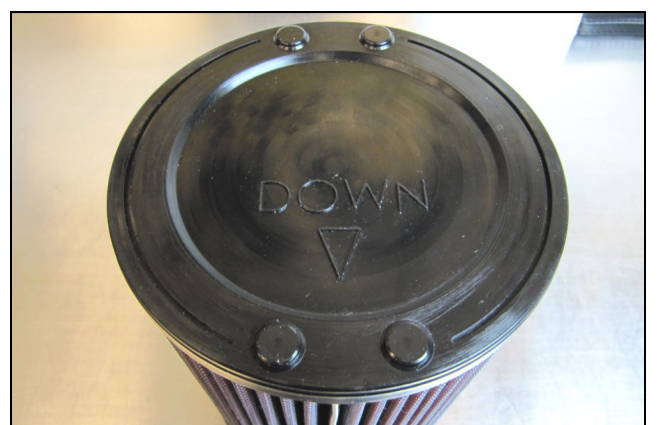
6. Notice that the Airaid Filter top has a directional arrow in the center and locating lugs in the 12:00 and 6:00 positions.
