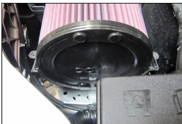
7. Install The Airaid Premium Filter (#1) and clamp into the air box as shown, with the Arrow pointing Down and the Lugs in the correct position. When properly installed, the Filter top will be completely inside of the airbox lower half.
