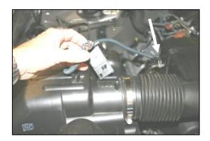
1. Stage I Disconnect negative battery cable. Remove 2 screws and remove and set aside the Mass Air Flow sensor from the factory airbox. Unclip wire harness from intake tube. (See arrow)
