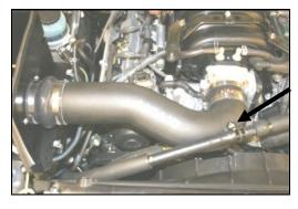
**17.** Install the MIT (#5) into the hump hose (#7), and then into the reducer (#6). Adjust the MIT snugly against the throttle body, and tighten all 4 hose clamps. Install the supplied button head bolt (#18), and washer (#19), thru the Adel clamp and into the MIT to hold the air conditioning hose.
