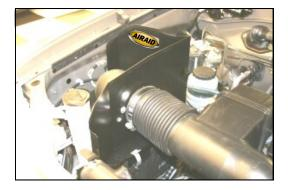
7. Slip MAF adapter into factory intake tube while installing CAD onto top of factory airbox. Adjust for fit, and latch 3 factory clips on factory airbox. Tighten the hose clamp on the intake tube. Replace the fan shroud bolt that was removed in step #5.
