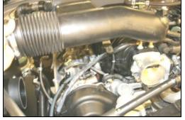
14. Remove the factory intake tube.
