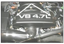
**13.** Remove two 10mm nuts, and the beauty cover from the top of the engine. Remove one bolt thru the Adel clamp that holds the air conditioning hose to the intake tube. Loosen hose clamps on each end of the factory intake tube.
