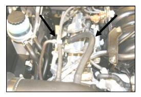
**18.** Install the vacuum tee (#13) into the 1/4"x4" hose (#14), and reconnect the factory 1/4" and 1/8" vacuum lines to the tee as shown. Install the 1/2"x13" breather hose (#8) onto the valve cover and to the MIT as shown.
