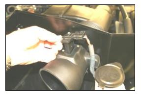
8. Re-route MAF wire harness under the intake tube, and around the front of the airbox. Install MAF sensor into the MAF adapter, using two supplied button head screws (#20). **DO NOT USE FACTORY SCREWS!**
