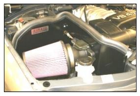
**8.** Install the Airaid Premium Filter (#1) onto the **MAF** adapter. Next install the weather strip (#10) on top of the **CAD**. Start at the radiator end and work you way towards the back.
