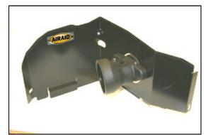
**3.** Assemble the Airaid Cool Air Dam (CAD) panels (#2, #3) using three 6-32 x 5/16" screws (#17), #6 flat washers (#18), and 6-32 keps nuts (#19). Install the MAF adapter (#4) using two 1/4 - 20 button head bolts (#20), and 1/4" flat washers (#21). Apply the Airaid Foil Decal onto the Panel as shown.
