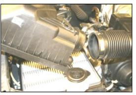
**2.** Unlatch the 4 clips on the factory airbox, and remove the lid. Remove the factory air filter.
