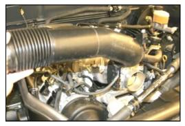
12. Remove the factory intake tube.
