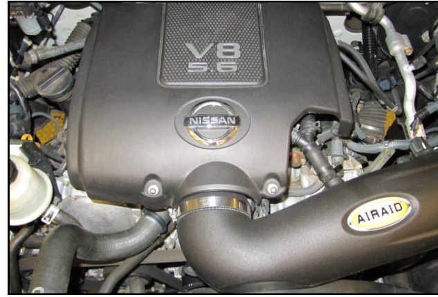
17. Reinstall the engine cover in the reverse order in which it was removed, rear first, front last. Only now it is to be secured using the two Acorn Nuts (#11) and two 1/4" flat washers.
