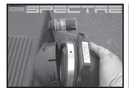
Step 6 Loosen the hose clamp securing MAF sensor to the air box. Carefully remove MAF sensor and rubber ring from the air box assembly and set aside for later use.
