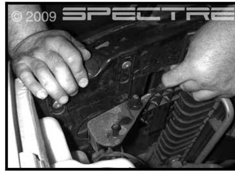
Step 8 Remove the plastic air box mounting bracket by sliding it upwards.
