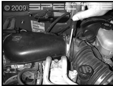
Step 5 Loosen air inlet clamp and remove stock intake assembly.
