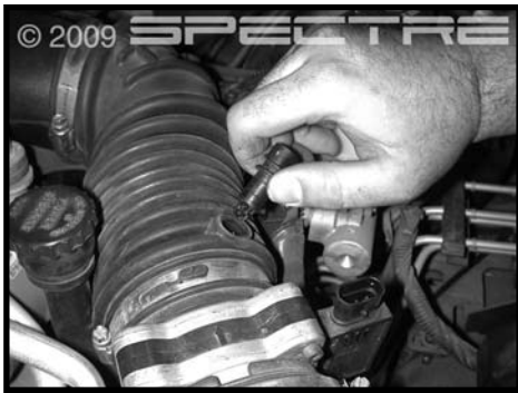
Step 4 Remove the IAT sensor from the stock rubber intake tube. Set the sensor aside for use later in the installation.
