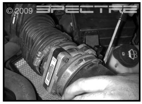
Step 6 Loosen clamps on both sides of the MAF sensor and carefully remove the sensor. Remove the rubber gasket from the air box side of the sensor.
