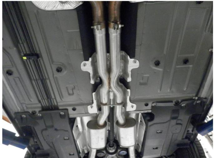
**Step 5.** With both valve assemblies cut from the OEM system, loosen the band clamps attaching the mufflers to the OEM tips. Both tailpipe sections may now be removed. Loosen the two OEM clamps at the outlet of the catalytic converters then carefully remove the rest of the exhaust system. Disengage all welded hangers from the rubber insulators. Do not discard or damage the clamps or rubber insulators as they will be needed to install the new system.
