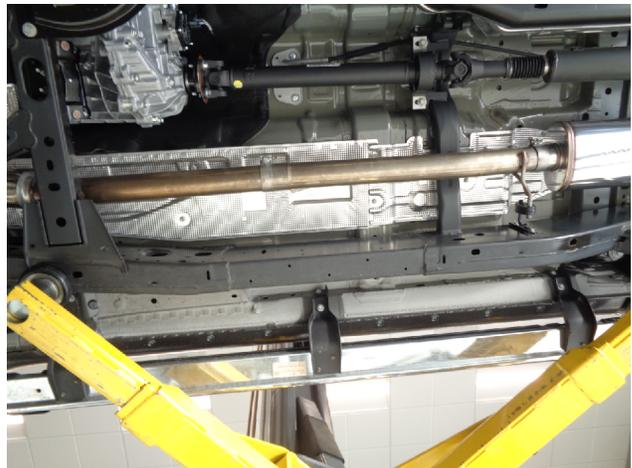
**Step 3.** Next, attach the Extension Pipe Assembly and the Muffler using the supplied 3.00" clamps and engaging the hanger into the rubber insulator.
