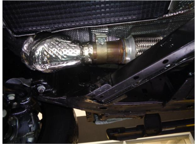
**Step 2.** Begin installation by attaching the Inlet Pipe Assembly to the outlet of the catalytic converter using the supplied 2.50" clamp and fitting the welded hanger into the rubber insulator (Leave all clamps and fasteners loose for final adjustment of the complete system.)
