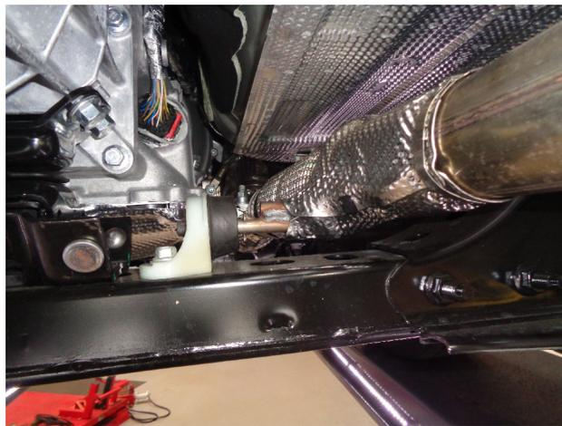
**Step 1.** To remove the OE exhaust system begin by loosening the clamps at the outlet of the catalytic converter and the inlet of the muffler. With the exhaust supported disengage the welded hangers from the rubber insulators and remove the system. Do not damage or discard the rubber insulators as they will be install the MagnaFlow system.
