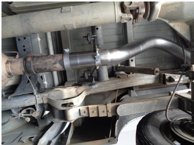
**Step 3.** Begin installation of the Magnaflow system by clamping the Inlet Pipe or Over Axle Pipe (depending on vehicle configuration) to the outlet of the DPF using a supplied 4.00" clamp. Locate the alignment notch to the OEM outlet. Slide the Hanger Clamp Assembly over the pipe and locate the welded hangers in the rubber insulators (leave all clamps loose for final adjustment of the complete system).
