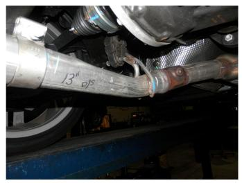
**Step 1.** To remove the OEM tail section of the exhaust you will need to carefully cut the OEM tail pipes. For the drivers side measure 13" rearward of the welded hanger brace behind the exhaust control valve as shown. Be Sure to deburr all cut edges.
