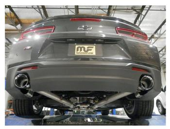
**Step 4.** Once a final position has been chosen for the new exhaust system, evenly tighten all clamps from front to rear using the torque specifications on page one of the instructions. Replace the shield and cross brace. Inspect all fasteners after 25-50 miles of operation and re-tighten if necessary.
