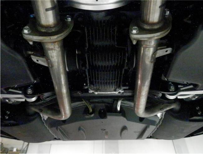
**Step 1.** Begin removal of the rear OEM exhaust mufflers by unbolting the two bolt flanges on each assembly at the resonator junction. Disengage all welded hangers from the rubber insulators. You may now remove both muffler assemblies. Do not discard or damage the OEM fasteners or rubber insulators as they will be used to install the new system.
