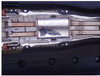
**Step 2.** Begin installation of the new system by loosely attaching the Resonator Assembly to the outlets using the 2.36" clamps. Leave all clamps loose until final adjustment.
