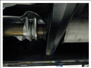
**Step 1.** To remove the OEM exhaust system, you will first need to unbolt the muffler assembly from the flange junction as shown.
