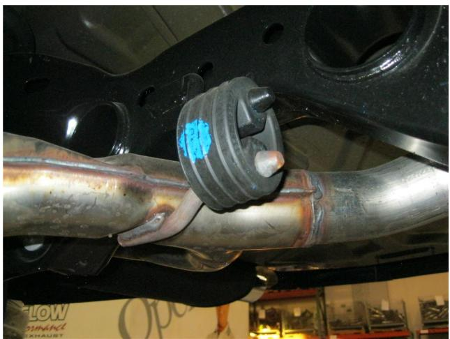
**Step 1.** To remove the OEM exhaust loosen the clamp located in front of the factory resonator. Next disengage all welded hangers from the rubber insulators (Do not damage or discard the rubber insulators as they will be re-used to mount the new system) and remove the exhaust from the vehicle.
