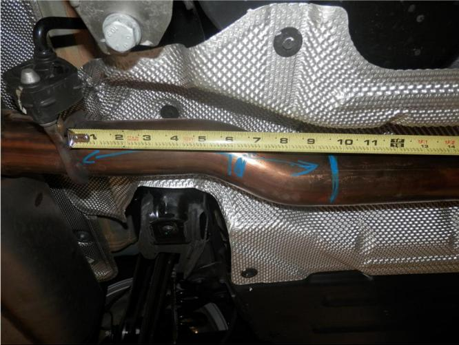
**Step 1.** Begin removal of the OEM muffler by cutting the exhaust pipe 10" forward of the welded hanger in front of the OE muffler as shown. Disengage the welded hanger from the rubber insulator and remove the muffler assembly. Deburr the cut pipe. Retain all OEM hardware as it will be needed to install your new MAGNAFLOW system.
