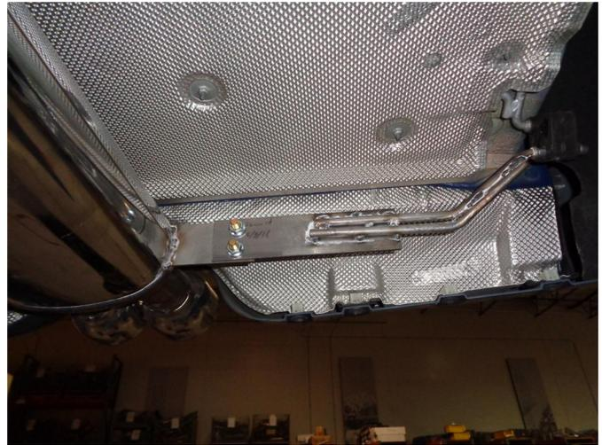
**Step 3.** Next, loosely install the Hanger Bracket to the bracket on the Muffler Assembly using the supplied hardware. Locate the hanger to the rubber insulator.
