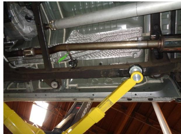
**Step 3.** Only the Crew Cab Long Bed configuration will require the supplied 12.5 Extension Pipe, Install this to the Inlet Pipe Assembly if required using the supplied 3.00" clamp then attach the Muffler Assembly to the Extension Pipe. If the 12.5" Extension Pipe isn't used attach the Muffler Assembly directly to the Inlet Assembly with a supplied 3.00" clamp.
