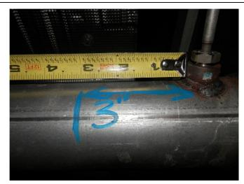
**Step 1.** Begin removal by removing the secondary O2 sensor at the over axle pipe of the OEM system. Next, cut the OEM inlet pipe 3.00" rearward of the O2 sensor behind the DPF.
