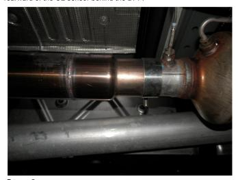
**Step 2.** There are two inlet pipe assemblies in the kit. 1. Wheelbase of 128.3" requires 6.5" Nipple. 2. Wheelbase of 140.5" requires 15.5" extension pipe and 6.5" Nipple. Begin installation of your new MAGNAFLOW system by loosely attaching the Inlet Pipe Assembly to the DPF outlet pipe you have just cut using the supplied 2.75" and 3.50" clamps. Engage the welded hangers to the rubber insulators. Reinstall the secondary O2 sensor.
