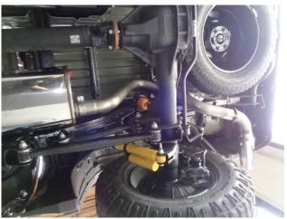
Step 2. Begin installation of the MagnaFlow system by attaching the Muffler Assembly at the two bolt flange using the supplied fasteners. Next, attach the Tail Pipe Assembly using the supplied 3.00" clamp and engaging the hangers into the rubber insulators. (Leave all clamps and fasteners loose for final adjustment of the complete system.)
