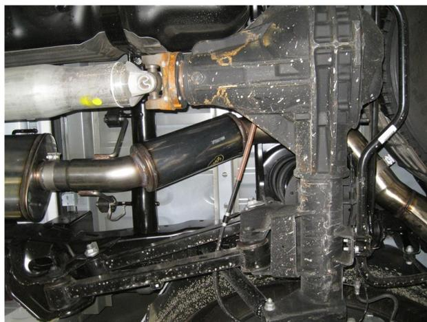
**Step 2.** Begin by attaching the Muffler Assembly to the factory outlet and the Resonator Assembly to the Muffler Assembly outlet using the supplied 3.50" clamps. Fit the hangers into the rubber insulators. Leave all clamps loose until final adjustment.
