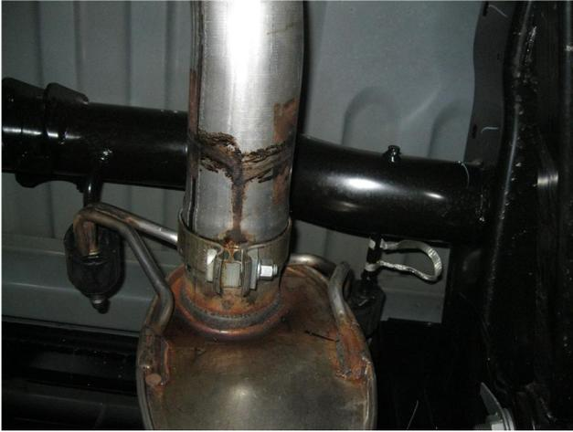
**Step 1.** Begin removal of the OEM system by unclamping the OEM Extension Pipe and muffler from the junction at the crossmember. You can then disengage the welded hangers from the rubber insulators, working rearward finish removing the system. Do not damage or discard the rubber insulators as they will be re-used to mount the new system.
