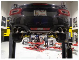
Step 4: Once a final position has been chosen for the new exhaust system, evenly tihgten all clamps from front to rear using the torque specifications on page one of these instructions. Inspect all fasteners after 25-50 miles for operation and re-tighten if necessary.
