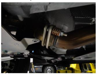
Step 2: Begin installation of the new system by loosely bolting the Inlet Pipe Assembly to the catalytic converter outlet using the supplied gasket and OE fasteners.
