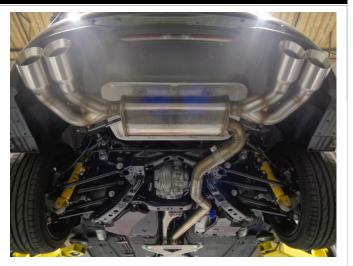
Step 3: Loosely attach the Mid Pipe Assembly to the Inlet Pipe Assembly using the supplied clamp. Locate the welded hanger to the rubber insulator. Loosely attach the Muffler Assembly in a similar fashion. Reattach both cross braces.
