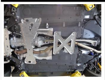
Step 1: To remove the OEM system you will first need to remove both cross braces shown. Unbolt the exhaust inlet from the catalytic converter at the flange junction. Disengage all welded hangers from the rubber insulators. The OEM exhaust may now be removed in one piece. Be sure to retain all mounting hardware as it will be needed to install your new MAGNAFLOW system
