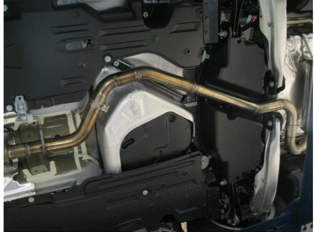
**Step 3.** Next attach the Mid-Pipe to the Resonator Assembly using a 2.50" clamp.
