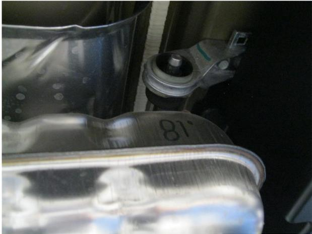
**Step 1.** Begin removal of the OEM exhaust by loosening the clamps located in front of the factory resonator and muffler assemblies. Working front to rear, disengage the hangers from the rubber insulators and remove the system. On this vehicle it may be easier to un-bolt the insulators from the frame rails. Do not damage or discard the rubber insulators as they will be re-used to install the new Magnaflow system.
