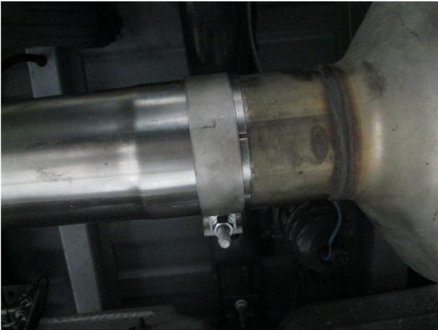
Step 1: Begin removal of the OE muffler by loosening the two clamps attaching the oe Muffler Assembly. Disengage the hangers from the rubber insulators and remove the muffler. Do not discard or damage the rubber insulators or rear clamp as they will be used to install the new system.
