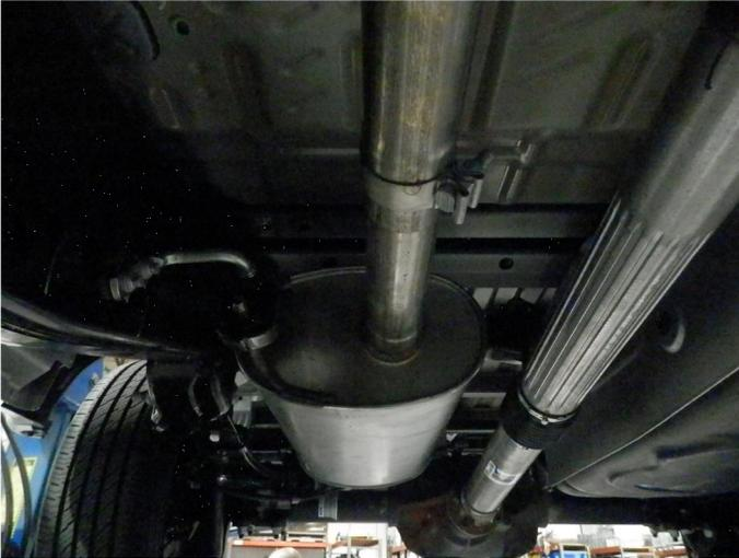
**Step 1.** The new exhaust system requires that you remove the spare tire from the vehicle. To remove the OEM exhaust system, loosen the clamp attaching the system inlet pipe to the resonator outlet pipe. Disengage all welded hangers from the OEM rubber insulators. Do not discard the OEM clamp or damage the rubber insulators as they will be needed to mount your new MAGNAFLOW system.
